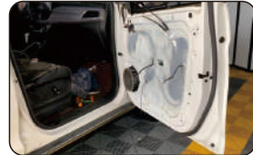
Open the door panel and directly remove it
