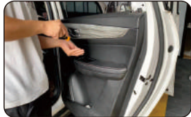
Open the car door and use tools to open the door panel
