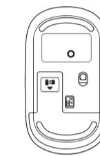
**Step 5: Insert the battery.(1xAA battery)**
