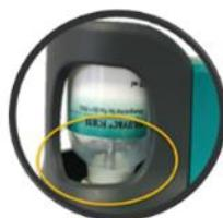
If '**Low Vial Warning**' is activated, the device will warn you once you can only perform 3 / 2 / 1 more vaccinations before the vial is empty (depending on your settings). You will also receive haptic feedback (if activated) and a corresponding warning symbol will be displayed next to each running pig.
