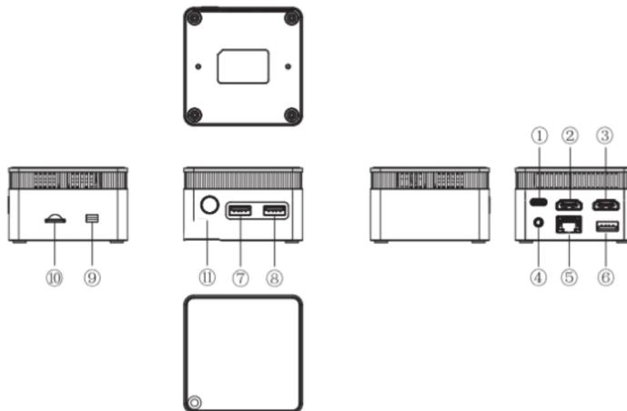
1, Power Input      2,HD Port      3,HD Port      4, Earphone      5, RJ45      6,USB3.2
