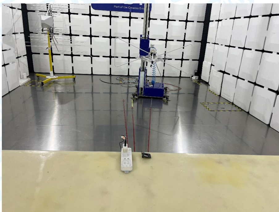
Photo of Setup for Radiated Emission (30MHz~1GHz)
