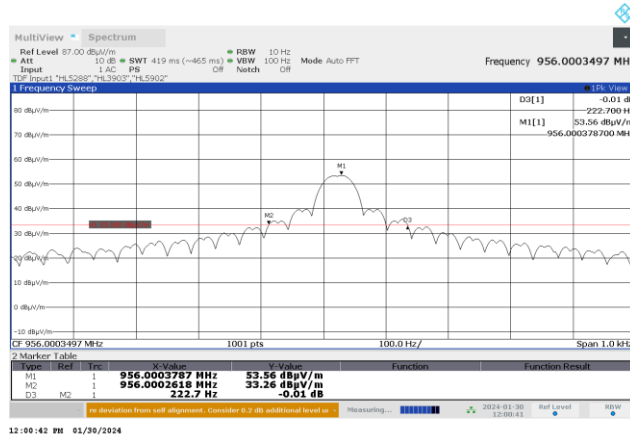
Plot 7.3.3 Occupied bandwidth test result at the fundamental frequency 956 MHz
