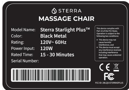
Specifications: The label shall be securely affixed to a permanently attached part of the device, in a location where it is visible or easily accessible to the user, and shall not be readily detachable. The label shall be sufficiently durable to remain fully legible and intact on the device in all normal conditions of use throughout the device's expected lifetime.
