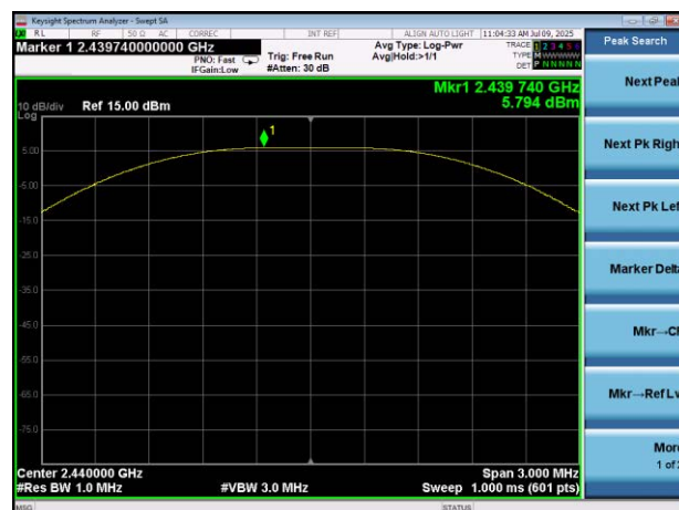
GFSK (BLE 1Mbps) MIDDLE CHANNEL
