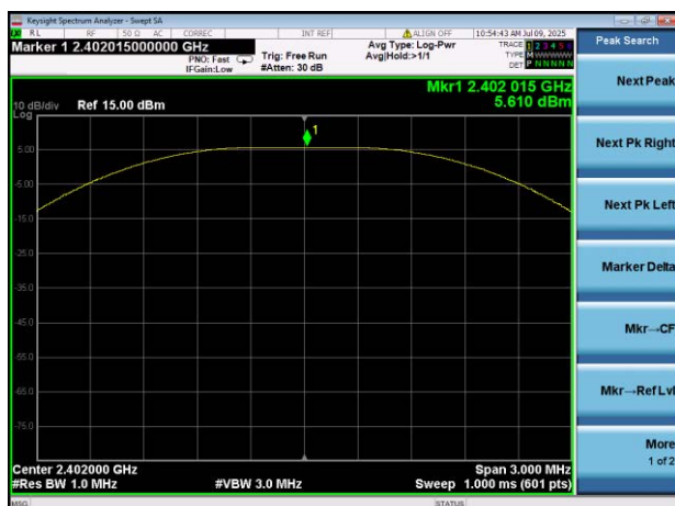
GFSK (BLE 1Mbps) LOW CHANNEL
