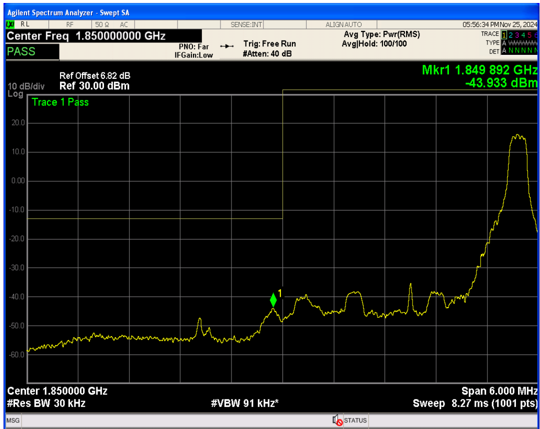
Band25 QPSK BW=3MHz Channel=26055 RB Size=15 Position=#0
