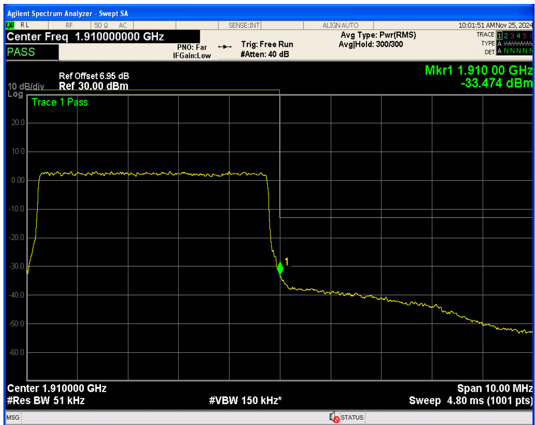
Band2 16QAM BW=5MHz Channel=19175 RB Size=1 Position=#Max
