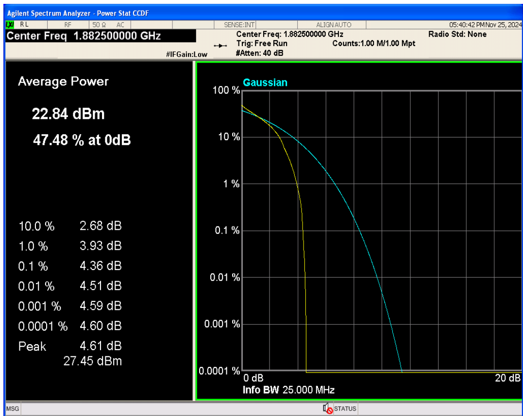
Band25 16QAM BW=20MHz Channel=26365 RB Size=1 Position=#0
