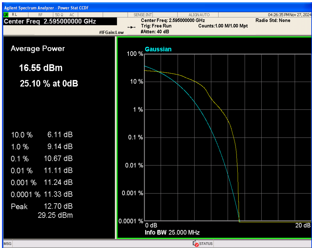
Band41 QPSK BW=15MHz Channel=40640 RB Size=1 Position=#0
