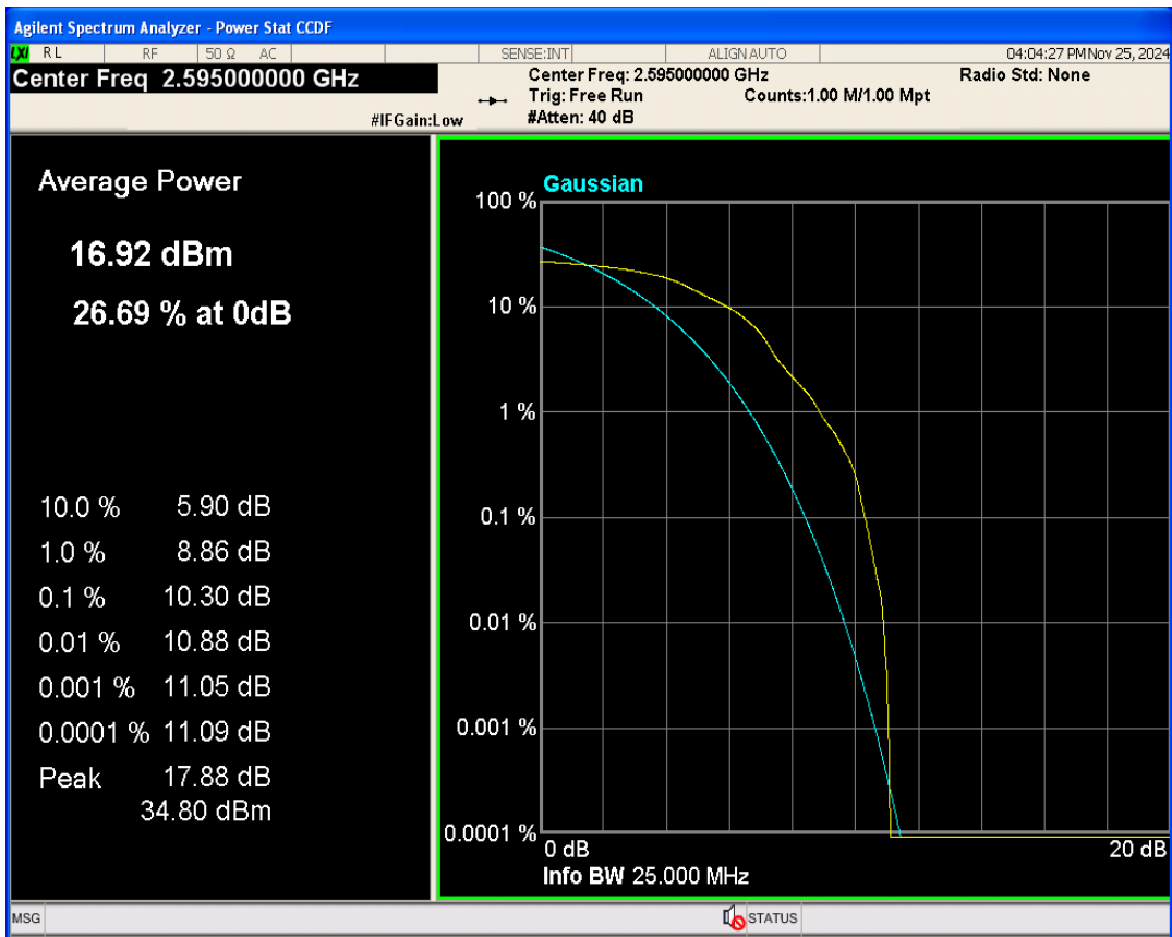
Band38 QPSK BW=10MHz Channel=38000 RB Size=1 Position=#0
