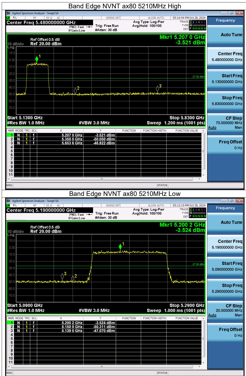
Note: A(B) Represent the value of antenna A and B. The worst data is Antenna A, only shown Antenna A
