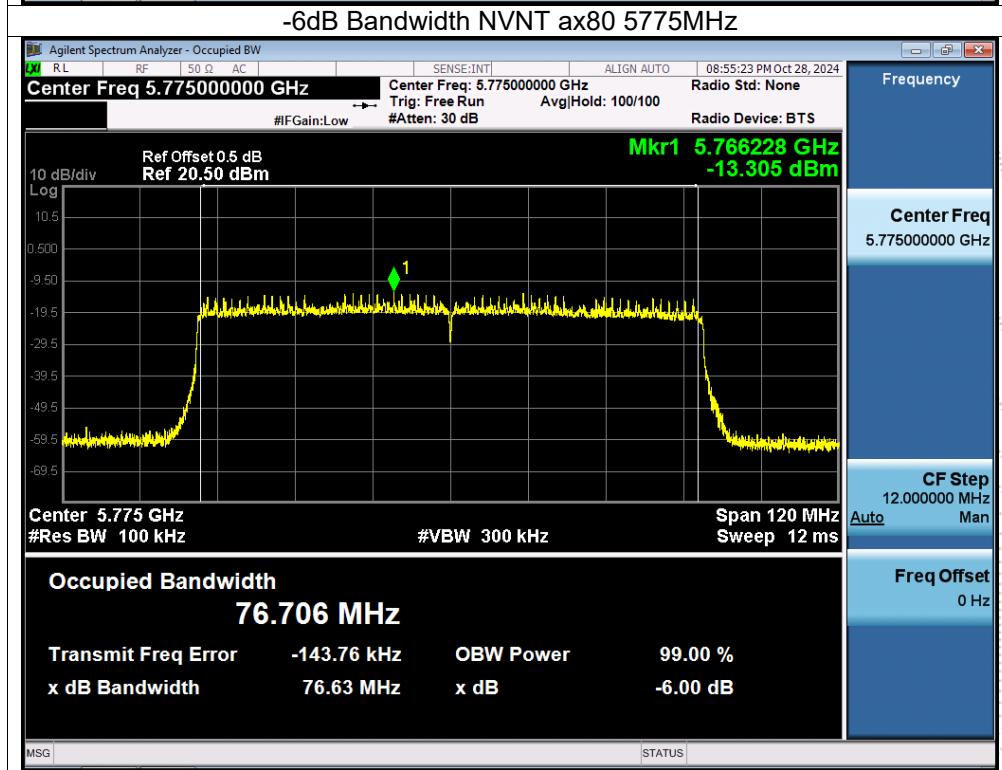
Note: A(B) Represent the value of antenna A and B, The worst data is Antenna B, only shown Antenna B Plot.
