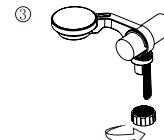
Insert the threaded strap through the locking hole and tighten via the included nut.
