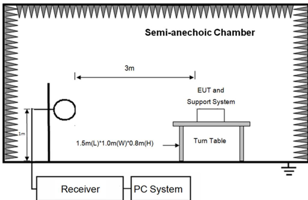
Test Setup Diagram for 30MHz~1GHz
