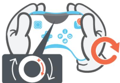
Rotate the right joystick to make the "cross icon" on the screen continuously rotate along the outer edge of the circle for 5 rotations.
