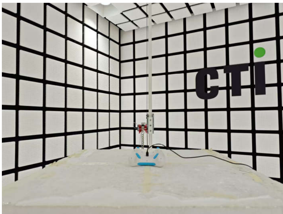
Radiated spurious emission Test Setup-2(Above 1GHz)
