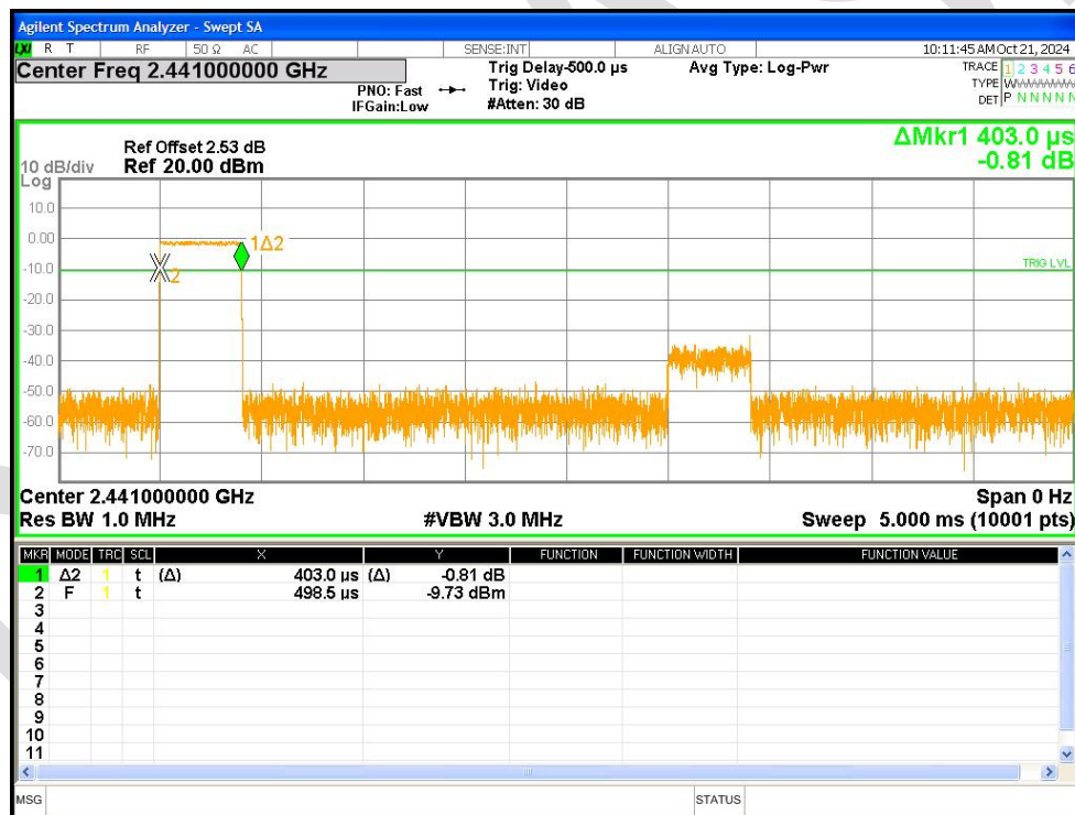
Dwell NVNT 1-DH1 2441MHz Ant1 Accumulated
