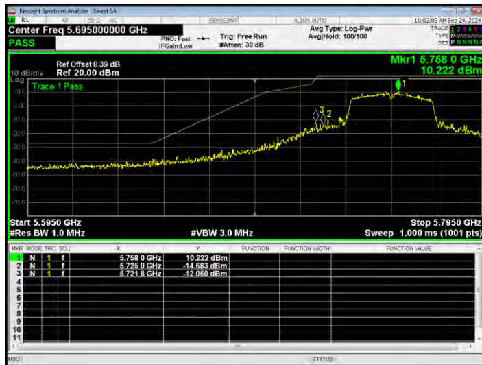
Band Edge NVNT ac40 5795MHz High Ant1
