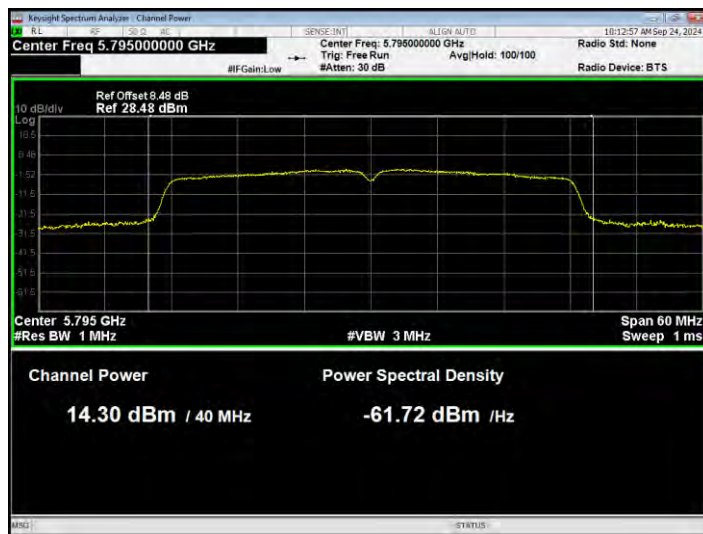
Power NVNT ax80 5775MHz Ant1
