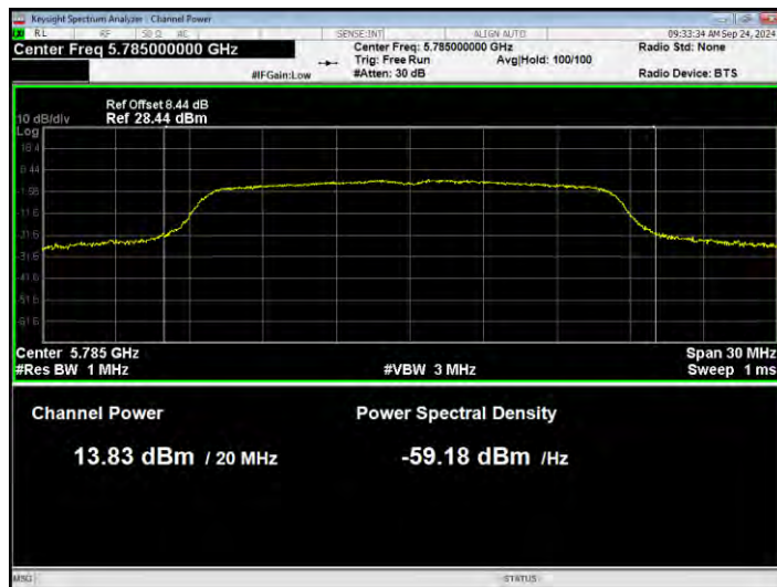
Power NVNT a 5825MHz Ant1
