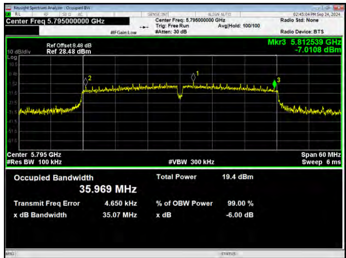
-6dB Bandwidth NVNT ac80 5775MHz Ant2
