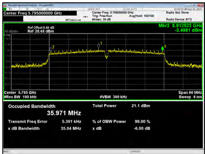
-6dB Bandwidth NVNT ac80 5775MHz Ant1
