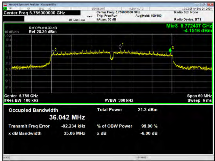
-6dB Bandwidth NVNT ax40 5795MHz Ant1
