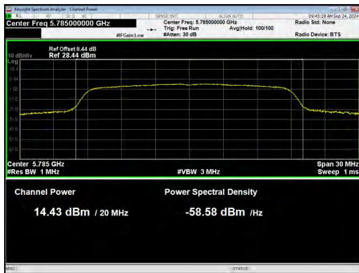
Power NVNT ac20 5825MHz Ant1
