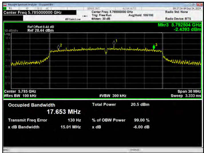
-6dB Bandwidth NVNT n20 5825MHz Ant1
