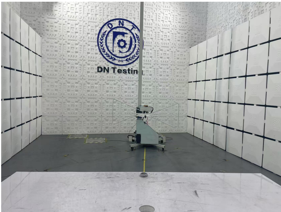
Radiated Emission Test View (Below 1G)
