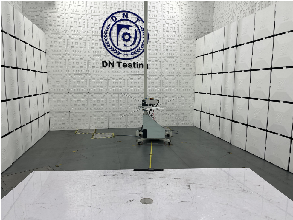
Radiated Emission Test View|(Below 1G)
