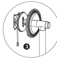
7. Before taking the display screen out of the package, first take out the trim ring at the back; then put the trim ring through the lifter.
