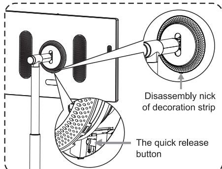
10. Align the locating hole of trim ring with the locating stud on the rear shell of the screen, and simply press to finish installation.
