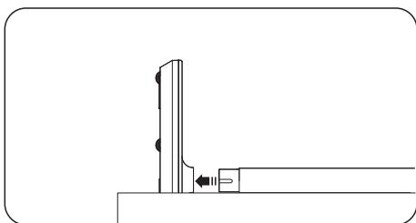
5. Install the lifter to the base by aligning it with the slot position.
