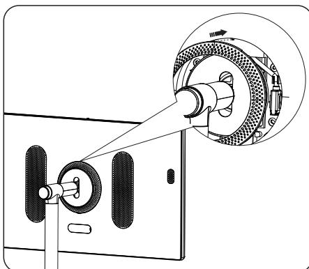
9. Wind power cable around the lifter clockwise, and insert power cable plug, then arrange power cable and clamp it into the buckle.
