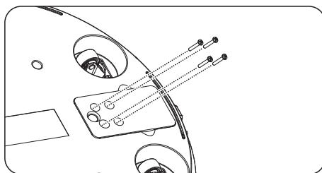
6. Align the screws with the screw holes, and then fasten the screws.
