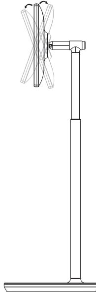
The height of the lifter is adjustable within  $190\pm10\text{mm}$
