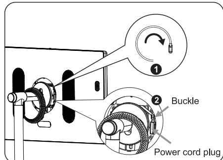
8. Tilt the display screen face up, and install it by alignment with the clipping position.
