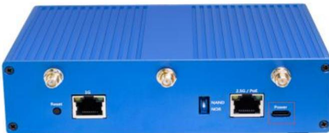
Use an Internet cable to connect to the WAN port of the device.
