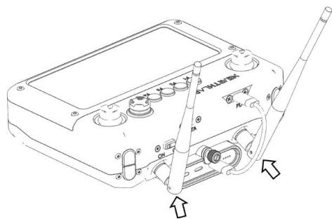
3. Press the power button for about three seconds to turn on.
