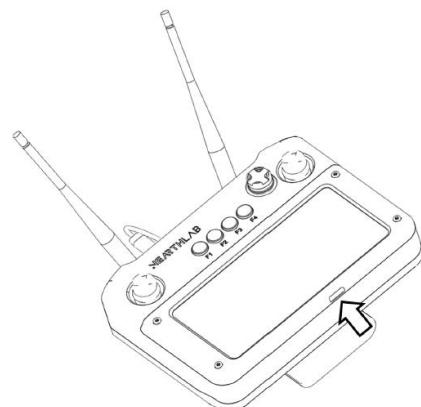
5. Turn the power toggle on at the top and check the ethernet device is recognized.
