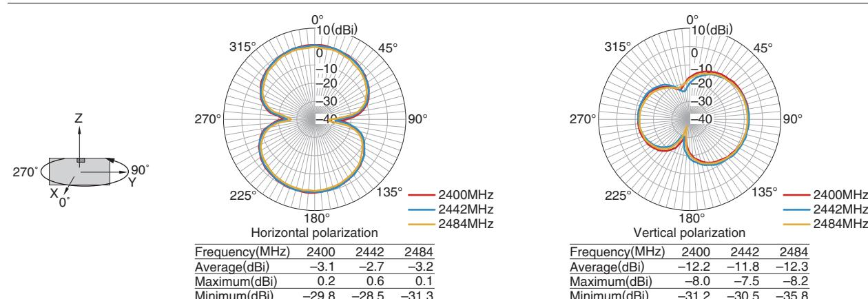
• Tested antenna has been soldered. Evaluation board size is 50x20x1 mm.
