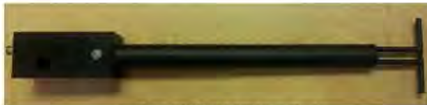
Figure 1 – MVG COMOSAR Validation Dipole
