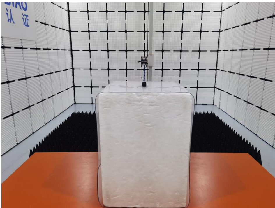
Radiated Emission Above 1GHz
