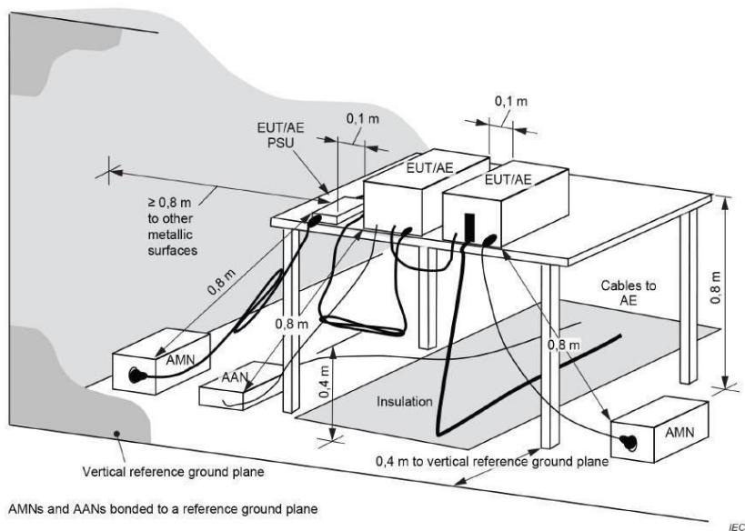
The LISN edge is arranged parallel to the edge of the test table
