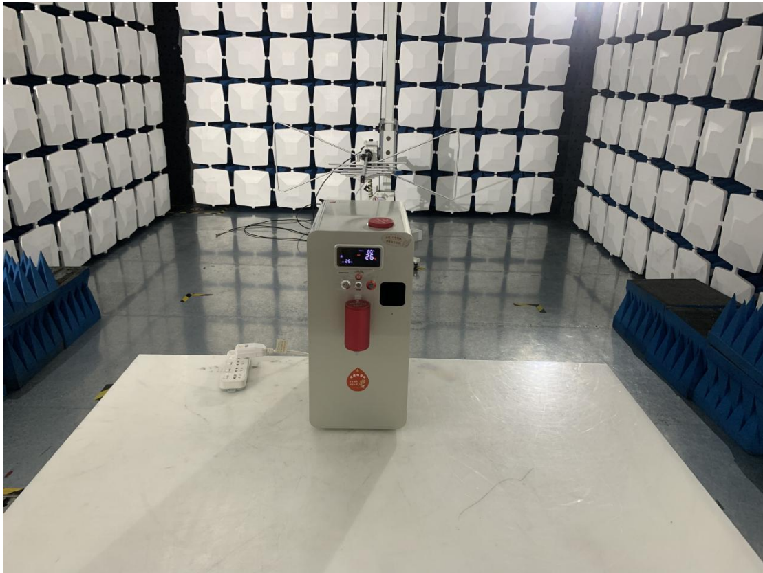
Below 1GHz for radiated emission test setup
