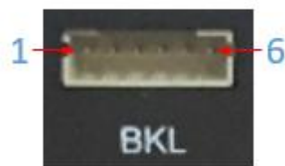
Figure 10. The LVDS backlight socket diagram
