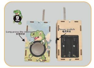
9. After the assembly is completed, refer to the above steps to assemble another walkie-talkie. (Turn on the power switch, press and hold the intercom button, you can talk, effective intercom distance: 50–100 meters, open areas up to 200 meters)
