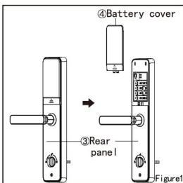
(1) As shown in Figure 1, remove the rear panel battery cover.
