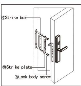
(6) As shown in Figure 6, place the door buckle box on the door frame, cover the door buckle box with the door buckle plate, and fix 4 buckle plate screws at the upper and lower ends.
