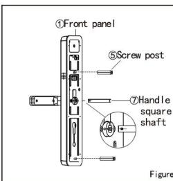
(3) As shown in Figure 3, fix the two screw posts to the front panel.
