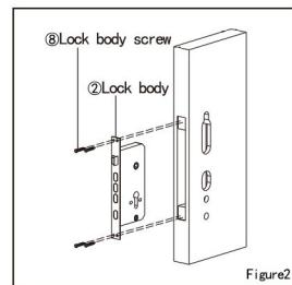
(2) As shown in Figure 2, install the lock body on the door and fix it with 4 screws.
