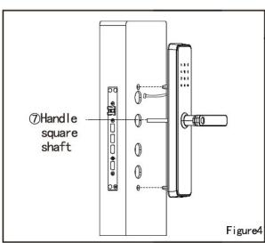
(4) As shown in Figure 4, pass the screw column, connecting line and square shaft of the handle on the front panel through the door.
