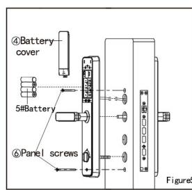
(5) As shown in Figure 5, connect the connecting line on the rear panel with the connecting line on the front panel, insert the corresponding square shaft into the handle hole, insert the locking pin into the locking hole of the lock body, adjust the panel position to align it, and fix the upper and lower panel screws. Install 4 No. 5 batteries and cover the battery back cover.
