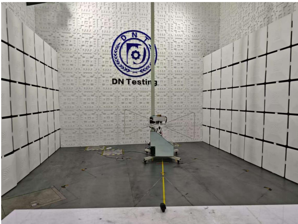
Radiated Emission Test View|(Below 1G)
