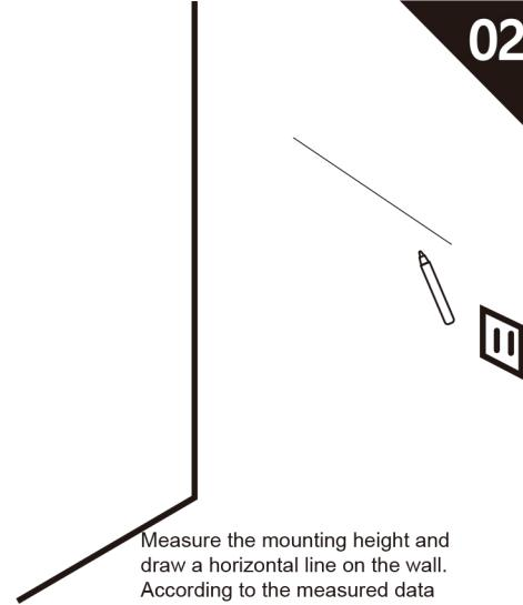
Measure the mounting height and draw a horizontal line on the wall.
