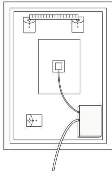
Measure the center distance between two hooks
