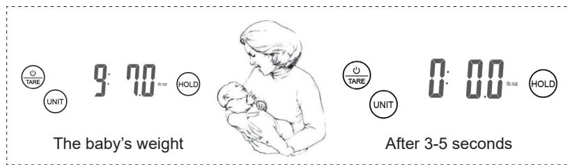
6.Notice: This scale has both automatic and manual "HOLD" functions. The auto HOLD function displays the weight when it has stabilized enough to detect an exact value.
