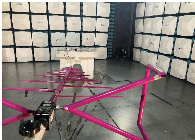
Photograph 9.2.1 Setup for final radiated emission measurements, general view
