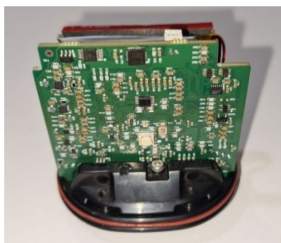
Photograph 11.2.2 Component side of the RF PCB
