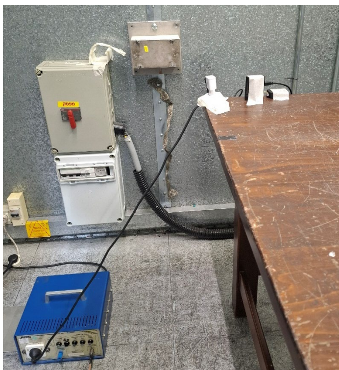
Photograph 8.6.1 Setup for conducted emission measurements
