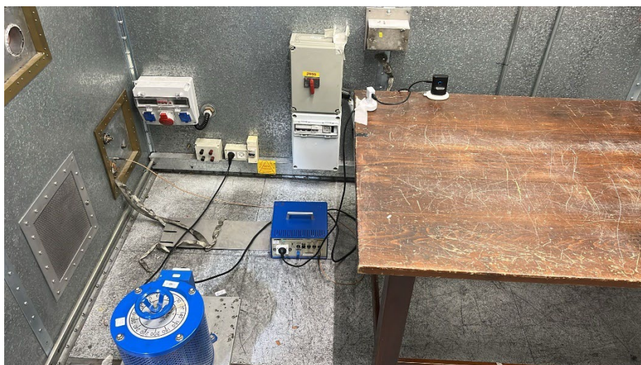
Photograph 9.1.1 Setup for conducted emission measurements
