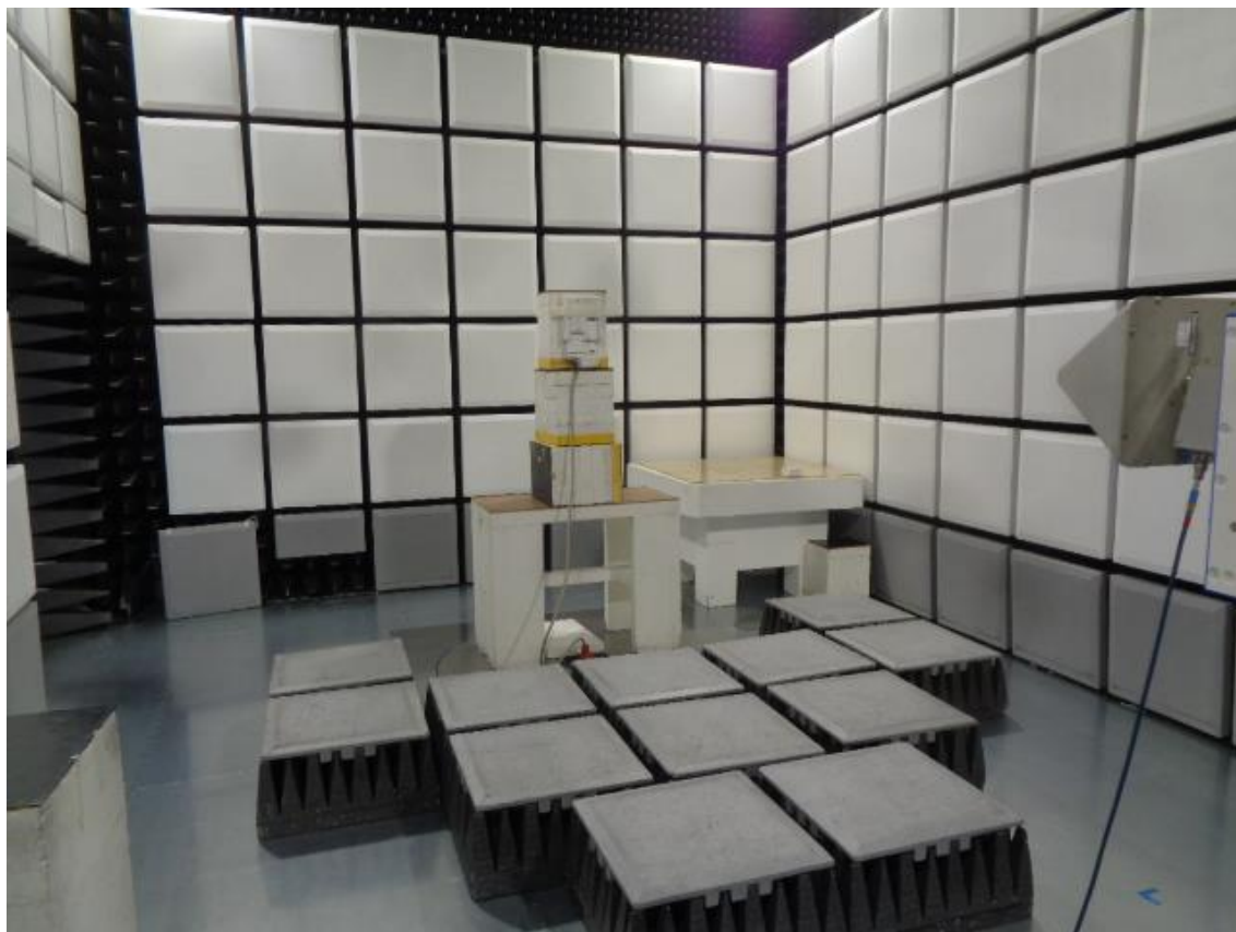
Figure 9.2-2: Radiated emissions above 1 GHz
