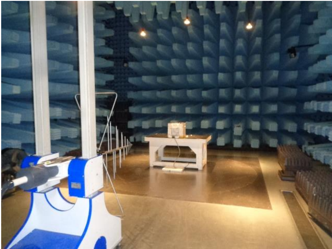
Figure 9.2-1: Radiated emissions below 1 GHz
