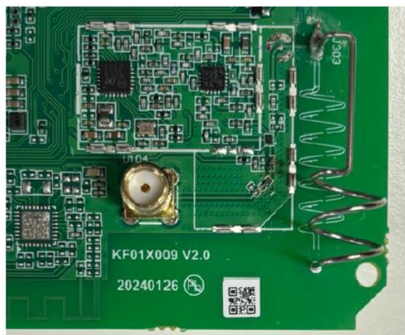
Figure 7- GLOBYSGNG3 radio module with internal antenna and without metallic shield
