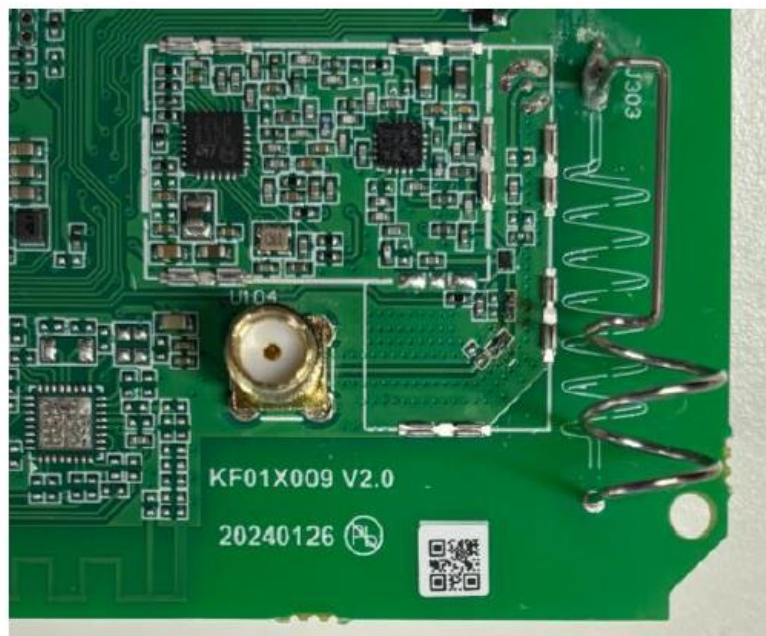
Figure 14 - GLOBYMGNG3 radio module with internal antenna and without metallic shield
