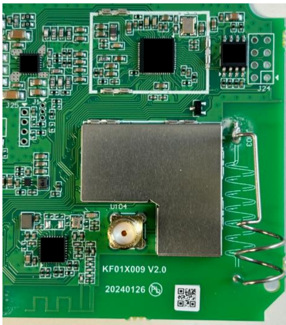
Figure 13 - GLOBYMGNG3 radio module with internal antenna
