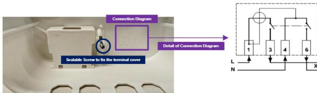
*The input/output terminals support cables with a cross section between 4 and 50 mm<sup>2</sup>. The fixing screws of the cables must be tightened with a torque of 6 Nm.*
