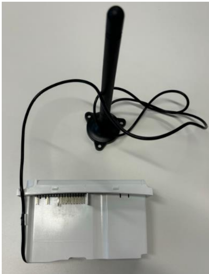
Figure 26 - GLOBYMGNG3 communication module with external antenna top side
