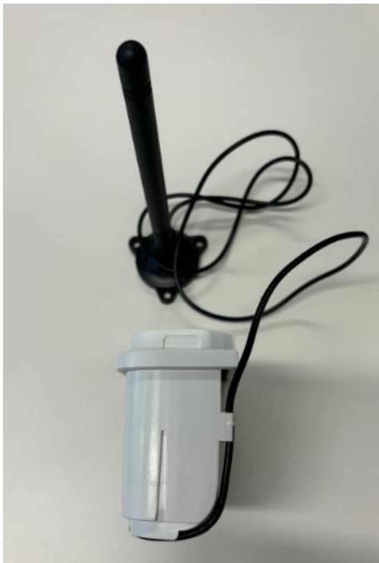
Figure 27 - GLOBYMGNG3 communication module with external antenna right side
