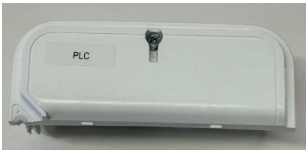
Figure 19 - GLOBYMGNG3 communication module with internal antenna front side
