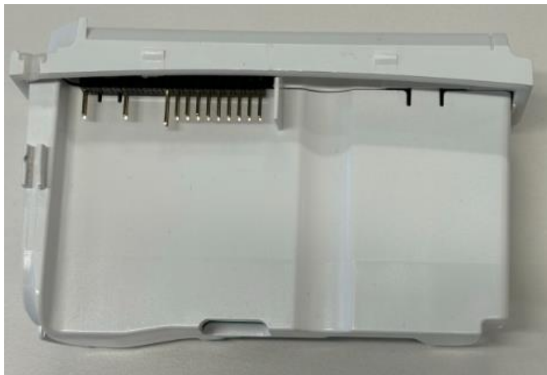
Figure 22 - GLOBYMGNG3 communication module with internal antenna bottom side
