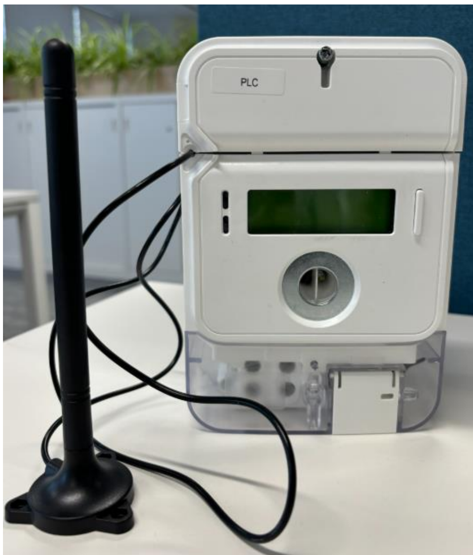
Figure 12 - GLOBYMGNG3 front side with external antenna basic version
