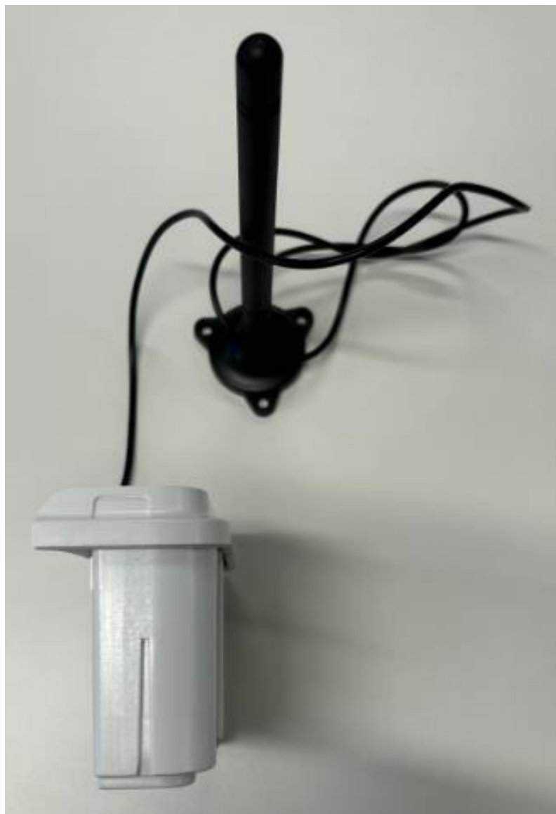
Figure 28 - GLOBYMGNG3 communication module with external antenna left side
