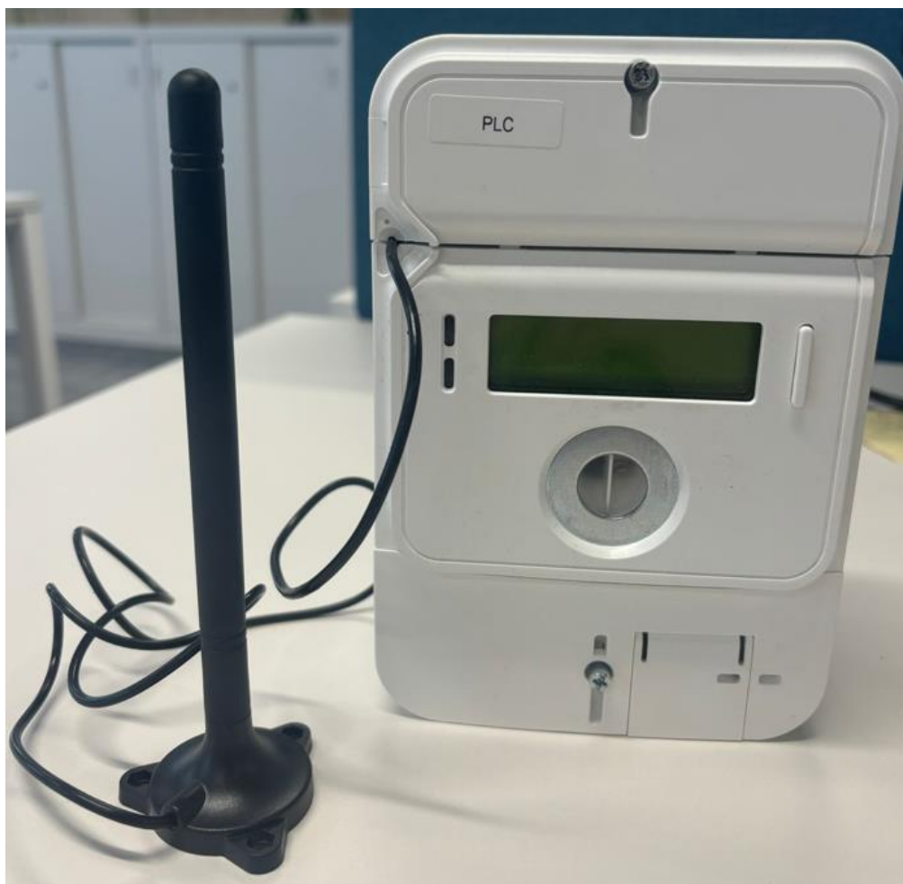
Figure 3-GLOBYMGNG3 front side with external antenna full version
