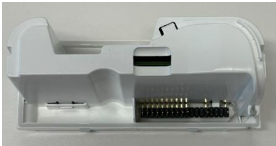
Figure 20 - GLOBYMGNG3 communication module with internal antenna back side
