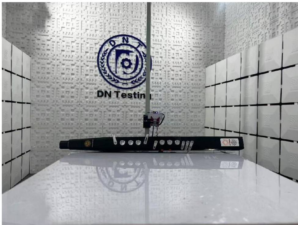
Radiated Emission Test View|(Above 1G)
