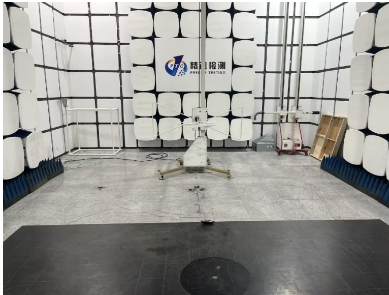
Radiated Spurious Emissions From 30MHz-1000MHz
