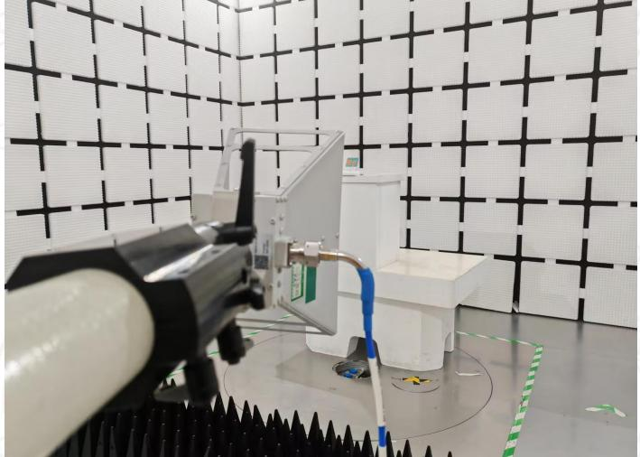
A photograph of a Faraday cage test chamber. A large horn antenna is positioned in the foreground, pointing towards a device on a turntable. The chamber walls are covered with a grid of black and white crosses.                                                                     |
