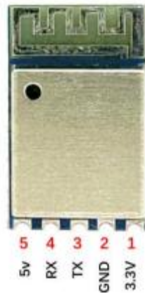
Figure 3 Pin Definition Diagram
