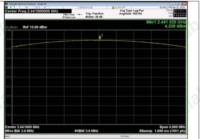
Peak Output Power 8DPSK_Channel 39
