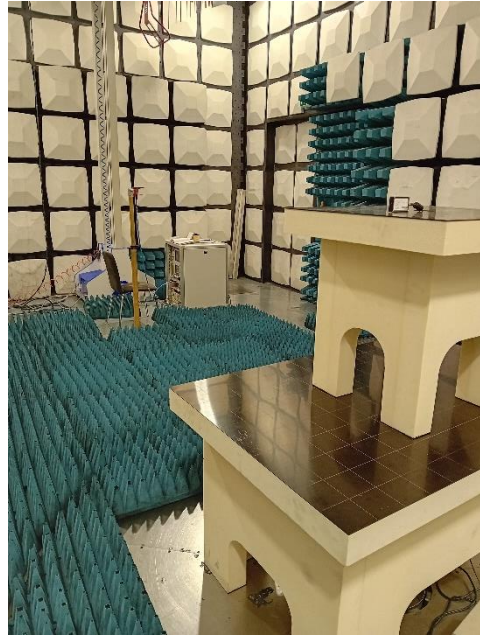
Test Setup – Radiated emission from 18 GHz to 25 GHz
