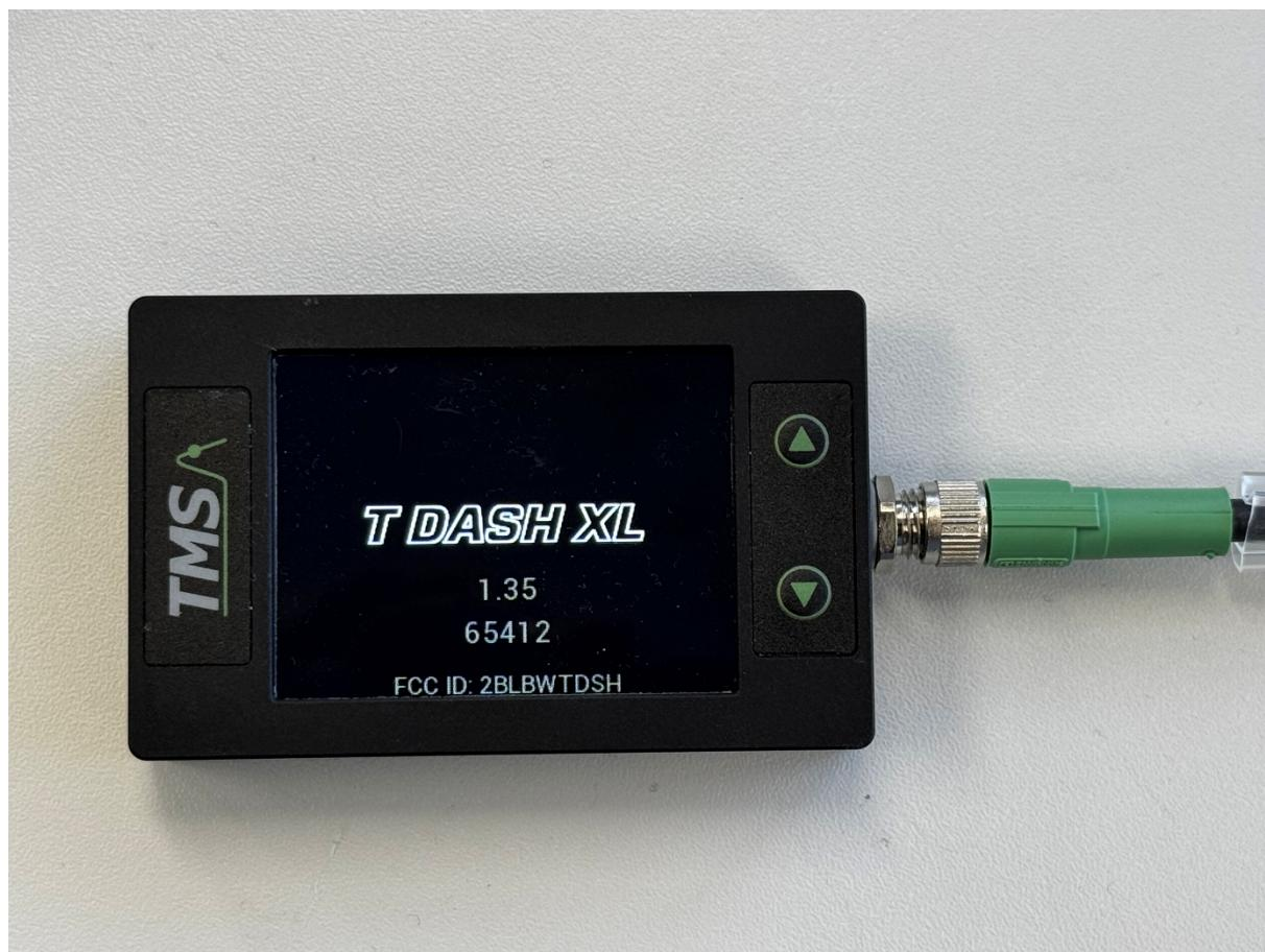
Label and Label location info: the FCC ID is displayed by e-labeling. The FCC ID is shown in the startup screen. The part 15.19 compliance text is placed in the user manual because it is impractical to place that on the device as the device is built in the back won't be visible to the user.
