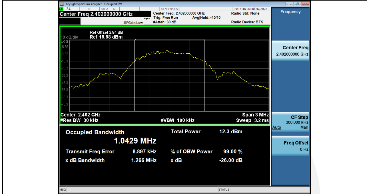
99% Occupied Bandwidth NVNT ANT1 1Mbps 2402
