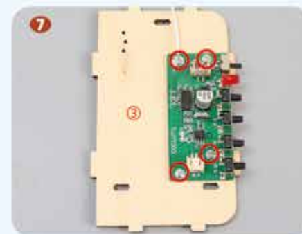
As shown in the picture, fix the circuit board on board No. 3 with screws
