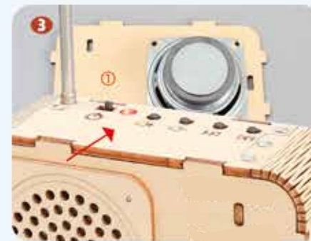
As shown, align the horn with the four small holes on board No. 1
